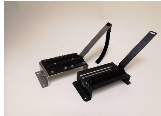
3D printed part and finished item in stainless steel
